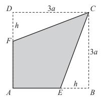
A uniform lamina AECF is formed by removing two identical triangles BCE and CDF from a square lamina ABCD. The square has side 3a and EB = DF = h (see diagram).
