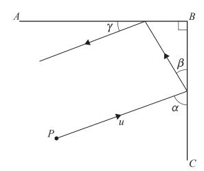
The smooth vertical walls AB and CB are at right angles to each other. A particle P is moving with speed u on a smooth horizontal floor and strikes the wall CB at an angle  $\alpha$ . It rebounds at an angle  $\beta$  to the wall CB. The particle then strikes the wall AB and rebounds at an angle  $\gamma$  to that wall (see diagram). The coefficient of restitution between each wall and P is e.
