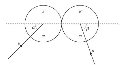
Two uniform smooth spheres A and B of equal radii each have mass m. The two spheres are each moving with speed u on a horizontal surface when they collide. Immediately before the collision, A's direction of motion makes an angle  $\alpha$  with the line of centres, and B's direction of motion makes an angle  $\beta$  with the line of centres (see diagram). The coefficient of restitution between the spheres is  $\frac{1}{3}$  and  $2\cos\beta = \cos\alpha$ .
