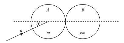
Two uniform smooth spheres A and B of equal radii have masses m and km respectively. Sphere A is moving with speed u on a smooth horizontal surface when it collides with sphere B which is at rest. Immediately before the collision, A's direction of motion makes an angle  $\theta$  with the line of centres (see diagram). The coefficient of restitution between the spheres is  $\frac{1}{3}$ .
